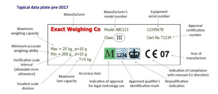
Newer equipment may also have some of the required markings indicated on the equipment's display screen rather than permanently displayed on the equipment body.
