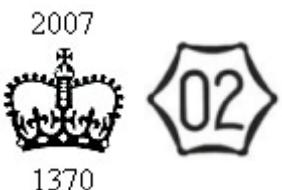
As with weighing equipment, any weights that bear a six-pointed star stamp were found to be inaccurate when they were last inspected and would be illegal for use for legal weighing purposes.
